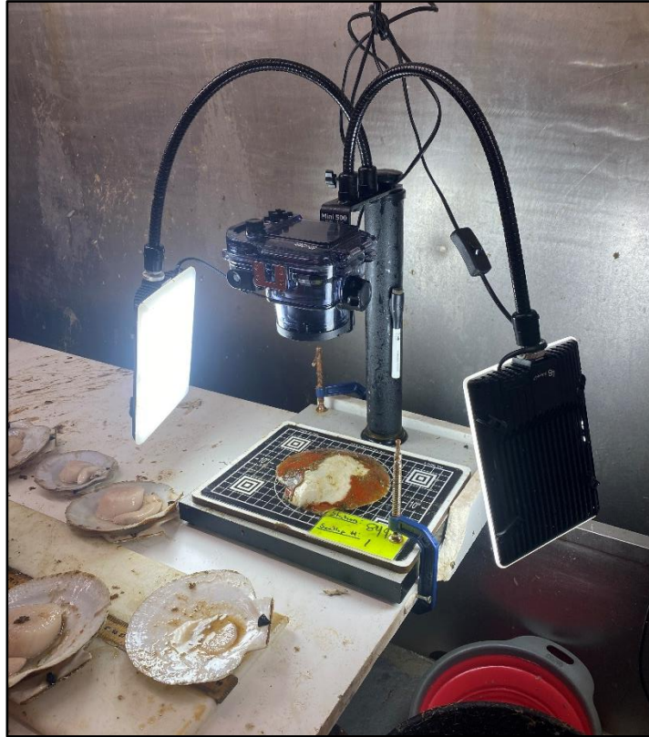
Figure 4. The camera station used to photograph scallop shells at sea for image annotation and subsequent epibiont analysis.
